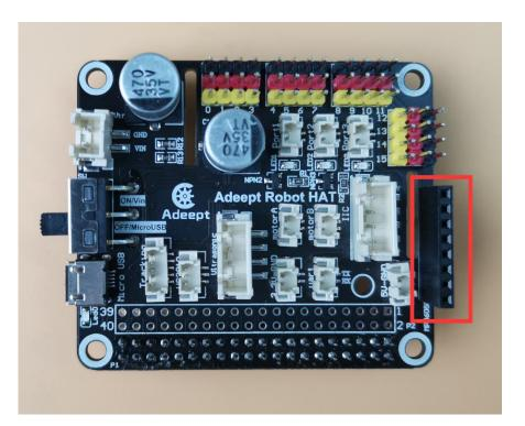
Only use the 4 pins below, from bottom to top: 3.3V, GND, GPIO03 (SCL1), GPIO02 (SDA1).
