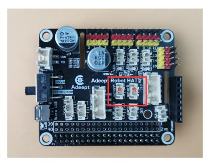
For the motor interface pins, the upper end is connected to the positive pole of the motor, and the lower end is connected to the negative pole of the motor.
