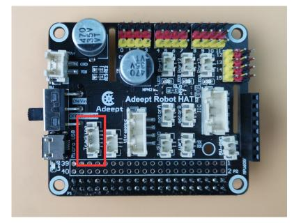
The pins of the three-way line inspection interface from top to bottom are: GND, GPIO19, GPIO16, GPIO20, 3.3V.
