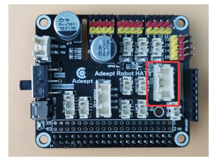
IIC interface pins from top to bottom are: 3.3V, GND, GPIO03 (SCL1), GPIO02 (SDA1).
