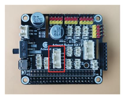
The ultrasonic interface pins from top to bottom are: GND, GPIO08, GPIO11, 5V.
