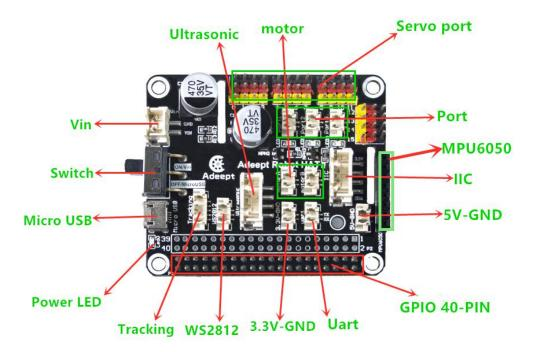
[Vin]: The vin interface is an interface for external power supply.
